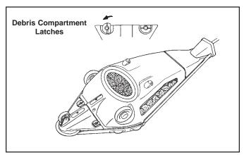
Figure 2. Open Debris Compartment Latches
